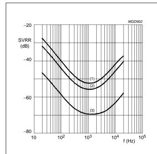
$\mbox{V}_{\mbox{CC}}$  = 7.5 V,  $\mbox{R}_{\mbox{L}}$  = 4  $\Omega,\mbox{R}_{\mbox{s}}$  = 0  $\Omega,$   $\mbox{V}_{\mbox{r}}$  = 100 mV.
