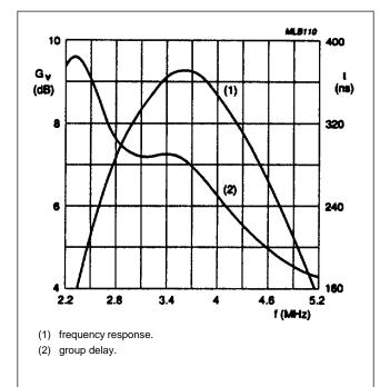
Fig.6 Band pass filter nominal frequency/group delay response (PAL mode).
