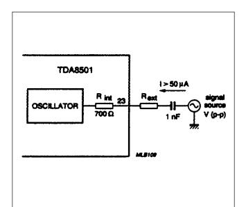
Fig.11 Tuning circuit for external signal source.
