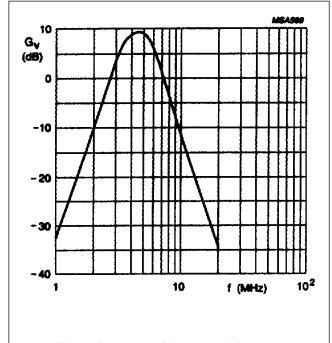
Fig.5 Band pass filter nominal frequency response (PAL mode).
