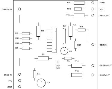
$\begin{array}{ll} R1 = 10\Omega \\ R2 = 220\Omega & 1/2W \\ R3 = 68k\Omega & 1/2W \\ R4 = 68k\Omega & 1/2W \\ R5 = 68k\Omega & 1/2W \\ R6 = 3k\Omega & R7 = 3k\Omega \\ R8 = 3k\Omega & R8 = 3k\Omega \end{array}$
