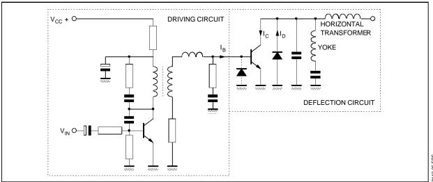
During the active deflection phase the collector current of the power transistor is linearly rising and the driving circuitry must be adapted to the required base current in order to ensure the power transistor saturation.
