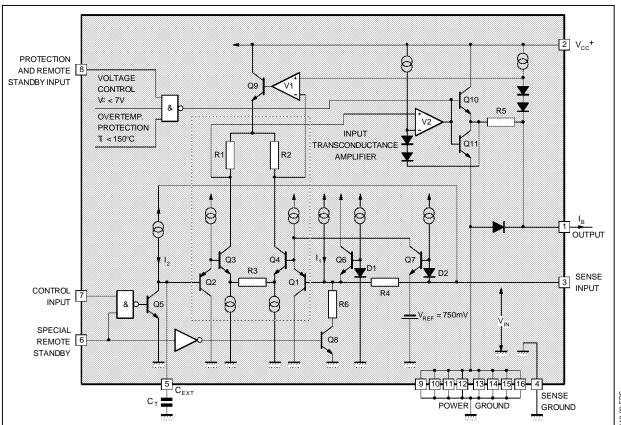
Figure 8: Integrated Horizontal Driver
