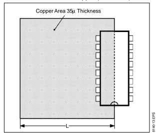
The presence of thermal shut-down circuit does mean that the heatsink can have a smaller factor of safety compared with that of a conventional circuit.
