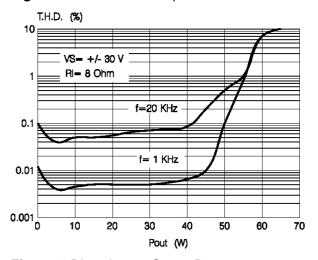
Figure 6: Distortion vs. Output Power
