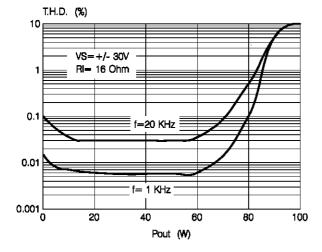
Figure 20: Distortion vs. Output Power
