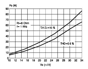
Figure 5: Output Power vs. Supply Voltage
