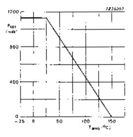
Fig. 2. Power derating curve.
