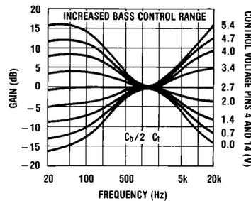
FIGURE 5. Tone Characteristic (Gain vs Frequency) TL/H/5142-8
