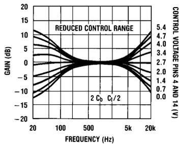
FIGURE 4. Tone Characteristic (Gain vs Frequency) TL/H/5142-7
