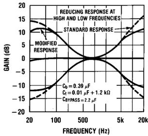
FIGURE 6. Tone Characteristic (Gain vs Frequency) TL/H/5142-9
